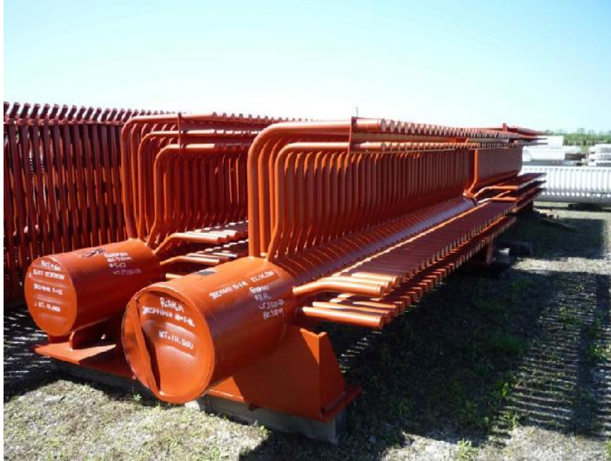
CFB BOILER HEADERS
