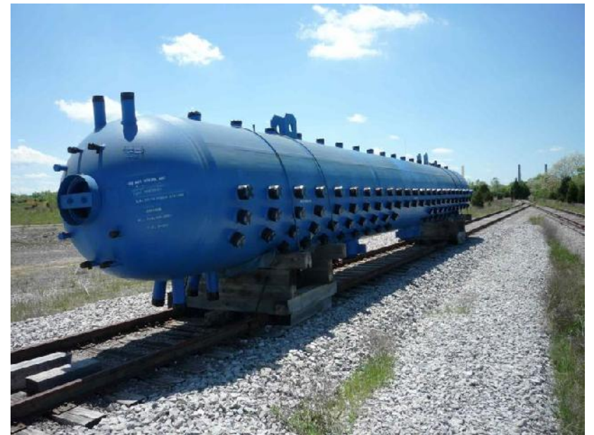
CFB BOILER DRUM
